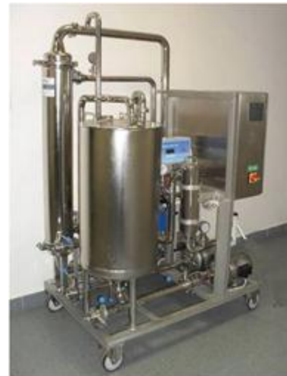
Figure 4: Photo of cross-flow microfiltration equipment
